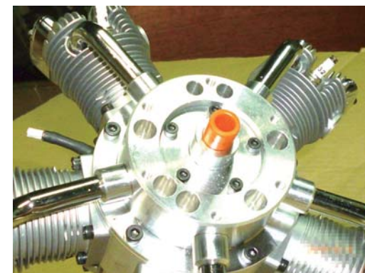
4. Detach the engine mount of Left side removing cap screws.
