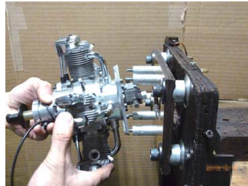
9. Put on the engine inserting 4 bolts in the mounting holes.
