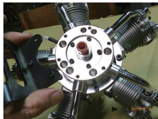
4. Detach the engine mount of Left side removing cap screws.
