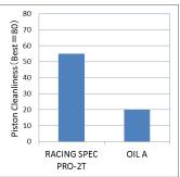
**2T engine test**: air-cooled 123cc engine, 7000r/min, full load, 3h, plug seat temperature 250°C,
